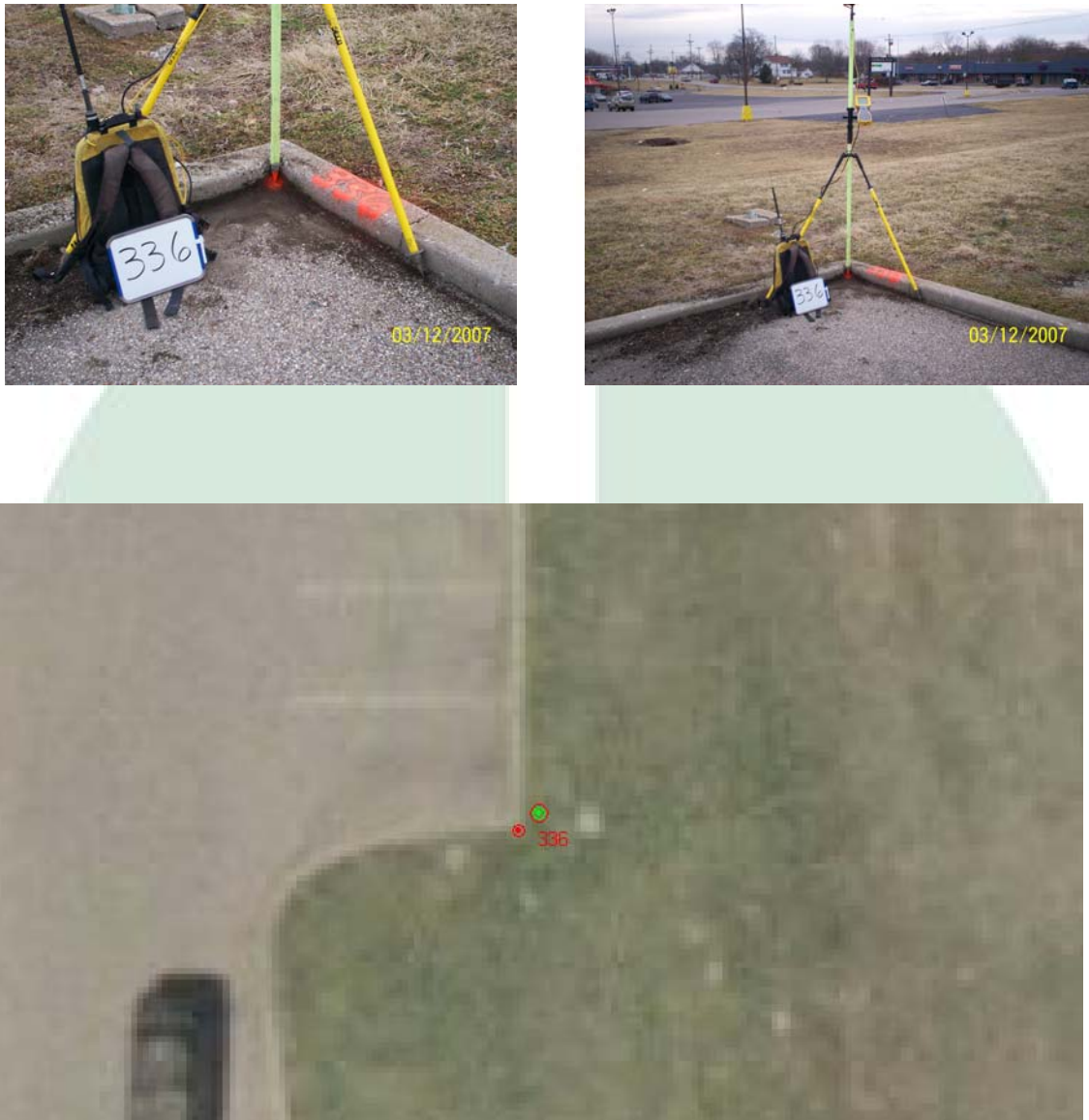
Figure 9. Optimal Checkpoint Location 336. The survey checkpoint (green) and photo identified locations (red) are shown.
